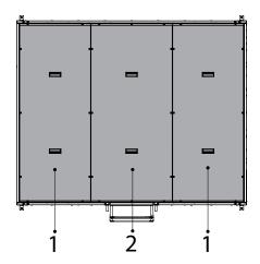
1: access panels for filters and fans (located at the bottom of the unit)
