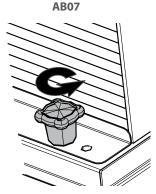
Remove the two butterfly bolts that fix the retaining clamp.
