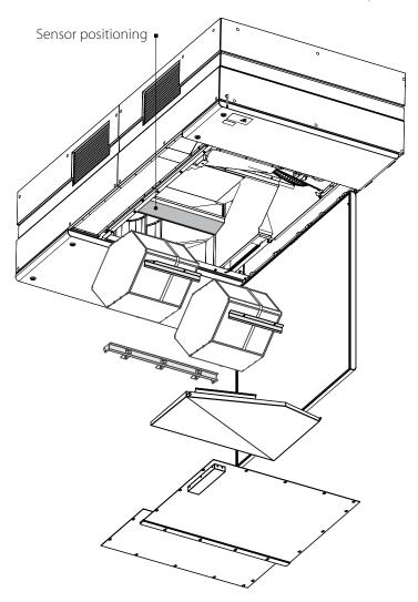
The CO2 sensor and VOC sensor are fixed on brackets. The humidity sensor is fastened with a threaded rivet.
