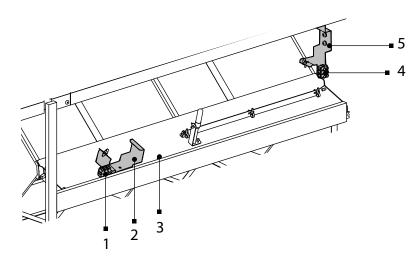
1 – terminal block of the CO2 sensor; 2 – bracket of the CO2 sensor; 3 – threaded rivet fixing place of the humidity sensor; 4 – terminal block of the VOC sensor; 5 – mounting bracket for the VOC sensor.
