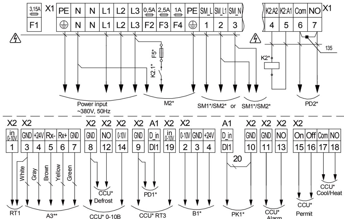
**MPA 700 E-3,0 EC, MPA 700 E-6,0 EC, MPA 700 E-9,0 EC,
