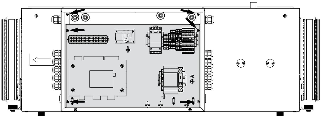
7. Connect all cables inside the unit in the new location at the same points as before disassembly. Reinstall the control unit cover.
