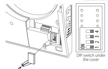
Prior to operating the ventilator set it up using the DIP switch. It is located on the controller circuit board.
