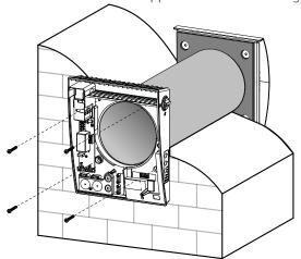
8. Route the power cable as figured below and connect the ventilator to power mains in compliance with the external wiring diagram, see section "Connection to power mains". Secure the power cable with the clamp.
