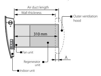
If the wall thickness is less than that in the layout of the blocks inside the wall, you can unfasten the fine filter holder and assemble the ventilator without it and without sound-absorbing material, as shown in the figure above.
