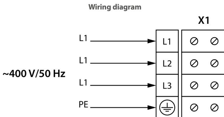
Connect the cables to the terminal block incorporated inside the terminal box located on the fan casing in compliance with the fan wiring diagram and the terminal designation. The terminal designations are shown on the label inside the fan casing. The electric parameters of the fan are shown on the label on the fan casing.
