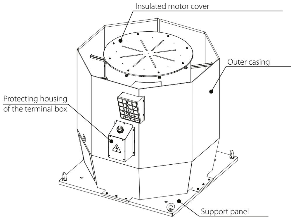
The roof-mounted smoke extraction fan consists of the welded support panel to which are attached:
