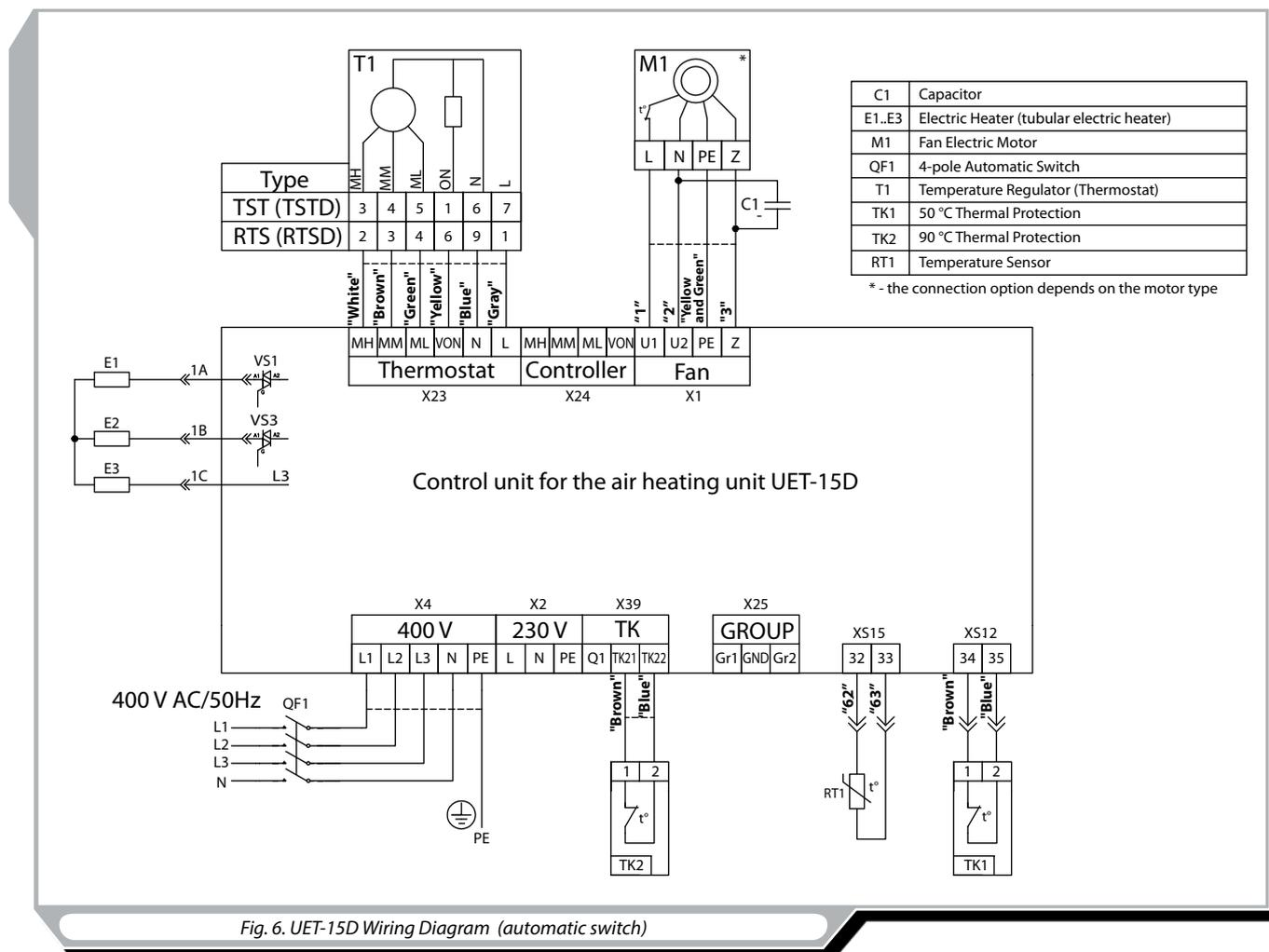
Fig. 6. UET-15D Wiring Diagram (automatic switch)
