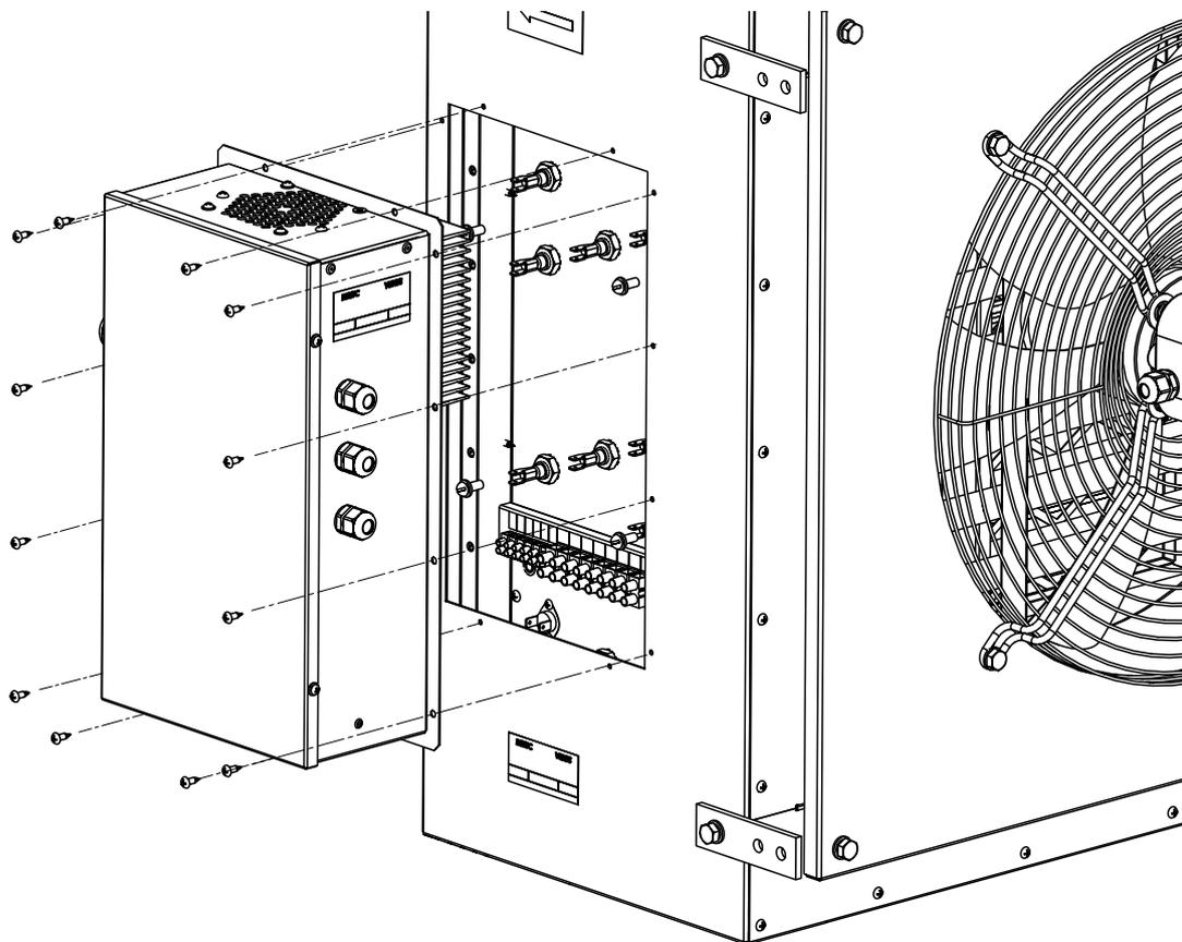
Fig. 3. Control Unit Installation
