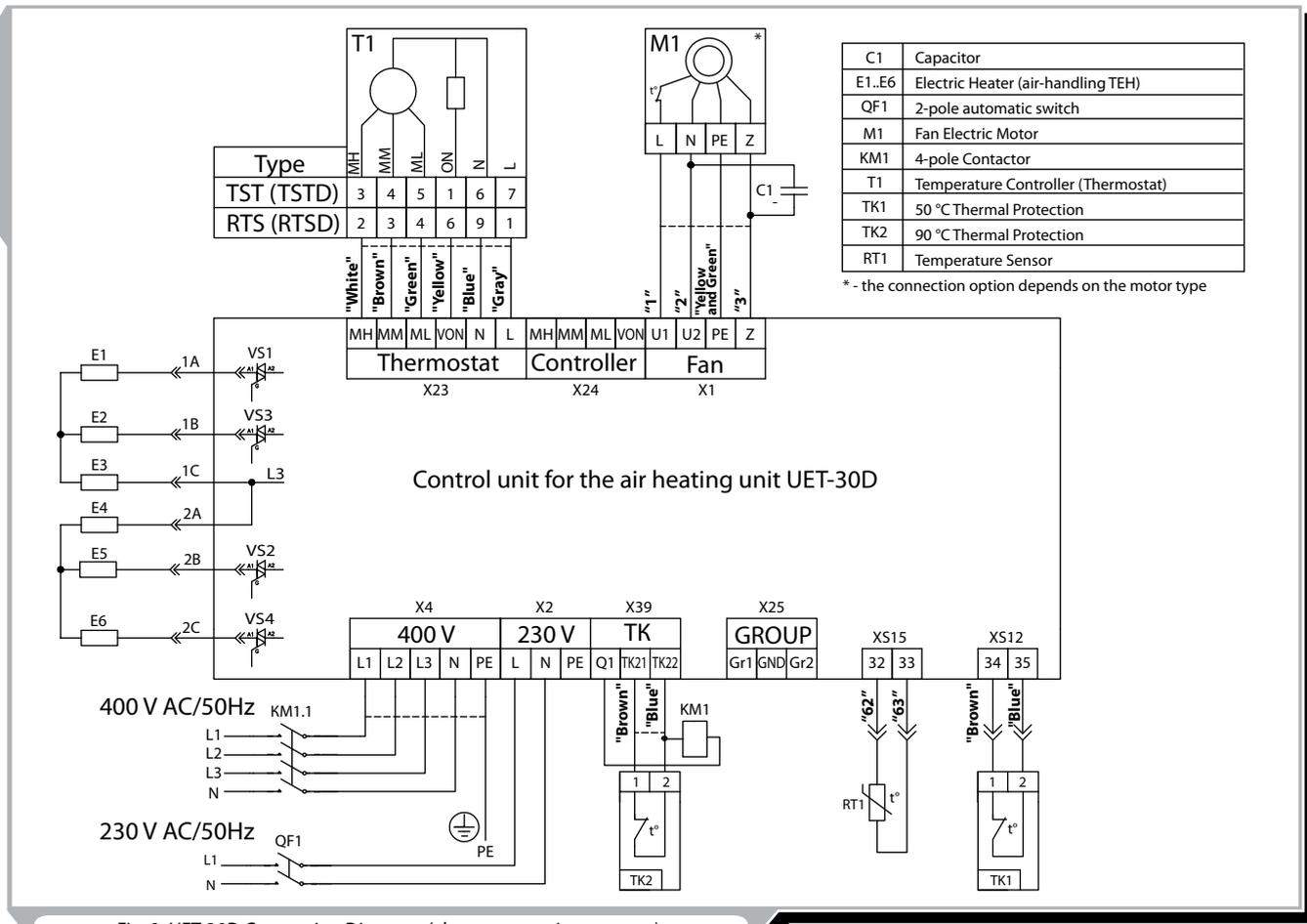
Fig. 9. UET-30D Connection Diagram (electromagnetic contactor)
