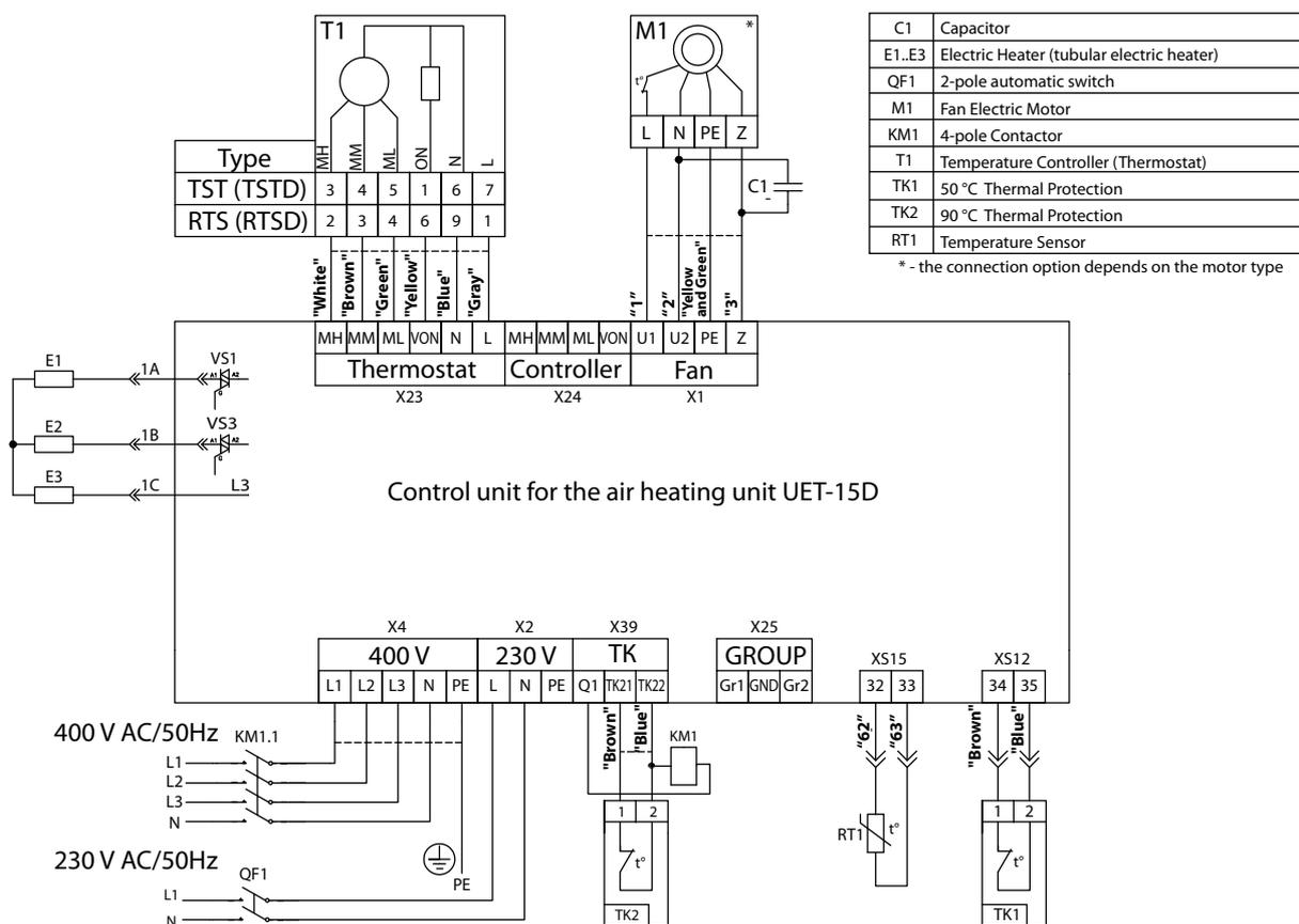
Fig. 7. UET-15D Connection Diagram (electromagnetic contactor)
