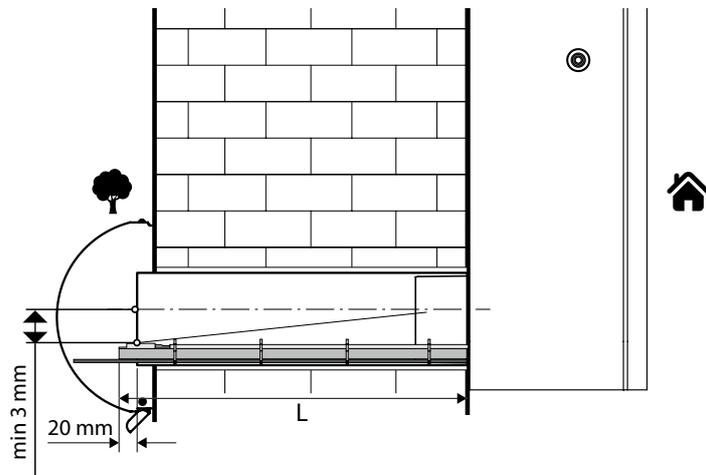
Mark the necessary length of the heater L on the guide tube, cut off the extra cable ties with wire cutters, move the cable away to the side and saw off the redundant part of the tube.
