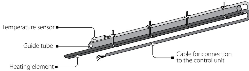
**1 Adjust the heater length L in consideration of the air duct length and the vent hood dimensions.**
